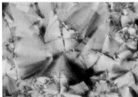
FIGURE 1 Optical polarized micrograph exhibited by smectic A phase of (n-Hexyl) 2 Tth. (See Color Plate VI).
